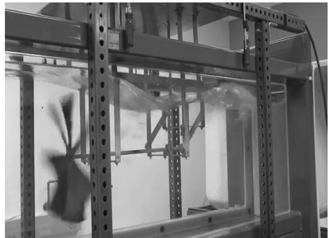
Fig. 10. A horizontal-axis hydrokinetic turbine with three blades under testing.
